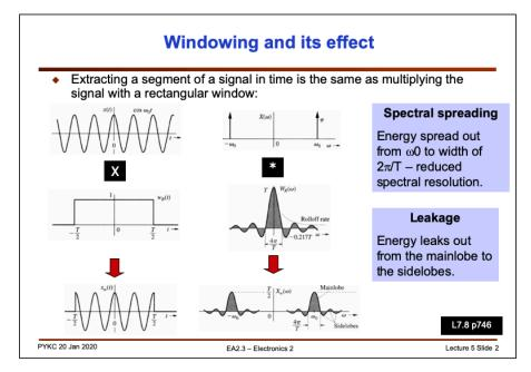
Extracting a portion of signal from an everlasting sinusoidal signal is the same as multiplying the everlasting sinewave with a rectangular function as shown.
