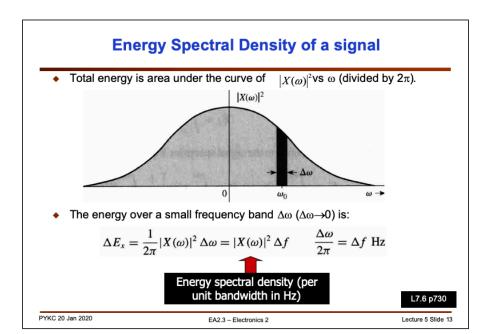
Therefore we can view the plot of  $|X(\omega)|^2$  as the energy spectral density of the signal. We can then ask the question: "how much energy is between two frequencies?" by integrating under the curve as shown.
